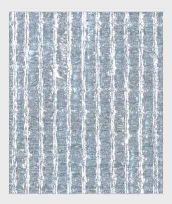
The Kalzip vapour layer FR should be applied parallel to the upper chords by peeling off the protective film on the underside. The longitudinal seams must be glued on the upper chords. Longitudinal and transverse seams must be sealed with a minimum overlap 8 cm by pressing or rolling. At all connections, terminations and penetrations the vapour barrier must be brought up to the upper level of the thermal insulation and sealed air- and vapour-tight.
