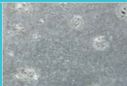
facing page: New plant Stile Bertone Caprie (I) Architect: Flavio Pacchioni left: Zinc, pre-exposed to weathering (macro-shot HCT-test 250 days) right: Kalzip AluPlusZinc®, produced by the PEGAL-process (macro-shot HCT-test 250 days)
