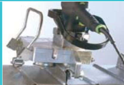
left: Kalzip® profiled sheets – lightweight and quick to install right: Kalzip® zipping machine
